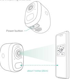
3) After a while, the camera will give out a prompt sound of a successful connection. At this moment, please set the name for the device on the App and select the location you want to place the device. Click "Done" to complete the pairing.
